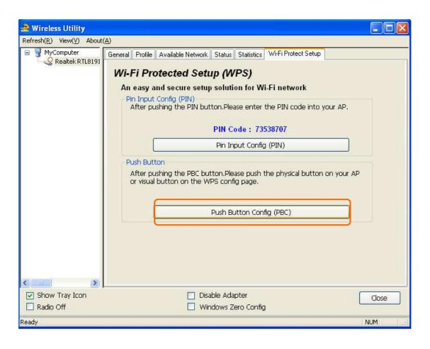
2. AU-4612 is waiting for the AP device to start the PBC function. The AP device PBC function should be started before AU-4612 WPS setup.
