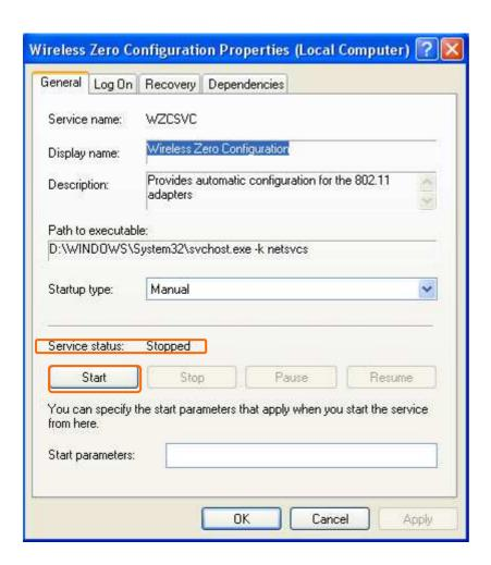
5. Once this setting is completed, the "Service status" is "Started". Click "OK" to finish and exit. Lastly, you will find the option of "Windows Zero Config" shown in AU-4612 Wireless Utility.
