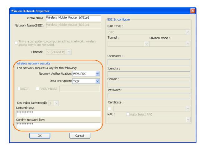
7. After finishing wireless network security section, please go back to "General" page to check the wireless network status. Once the wireless network is connected successfully, the Network Address will indicate AU-4612 IP address assigned from
