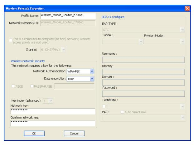
6. Wireless network security section: Please select the Network Authentication and Data encryption to set the encryption type.
