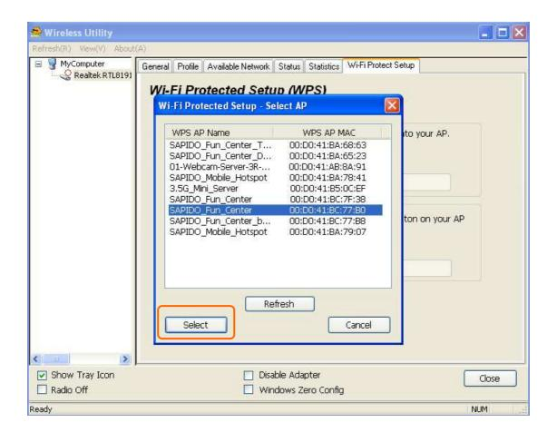
3. After selection, the specific AP will establish the connection with AU-4612 meanwhile you will get a PIN code (here example is 67382316) and you need to input this PIN code into the specific AP before initial WPS completes. For example,
