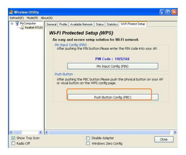
2. AU-4912 is waiting for the AP device to activate the PBC function. The AP device PBC function should be started before AU-4912WPS setup.
