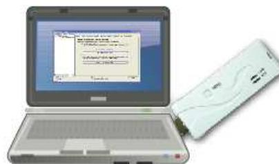
(2) Press the WPS button (A) from RB-1800 and wait for Wireless/WPS LED light (B) changed into red.
