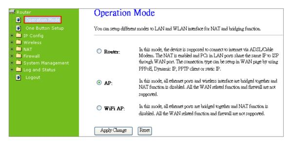
When this product is used as an access point, the IP address has to be changed. The default IP under AP mode is 192.168.1.254.
