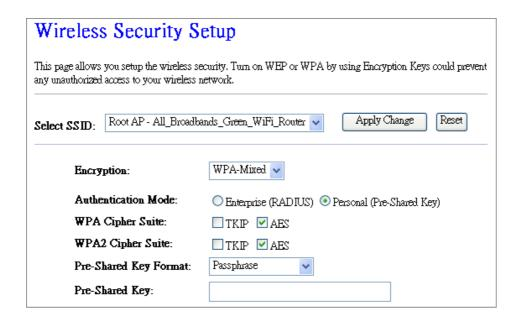
(3) Apply Change & Reset: Click on 'Apply Changes' to save setting data. Or click 'Reset' to reset all the input data.
