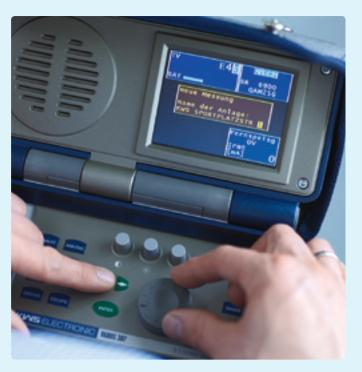
The name of the measurment place is given in – choose the channels and transponder where it should be measured – and start.
