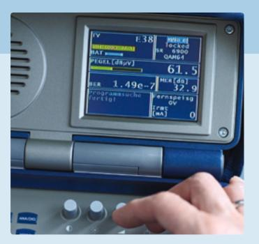
Easy and fast logging of measurments and functions on the PC with the measurment memory  ${\tt wVAROS.data}{\tt wC}$
