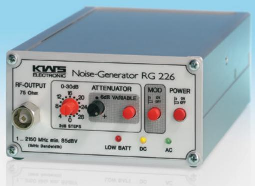
The Noise Generator RG 226 enables you to assess the frequency progressions of entire distribution systems as well as those of individual components such as amplifiers and multi-switches.
