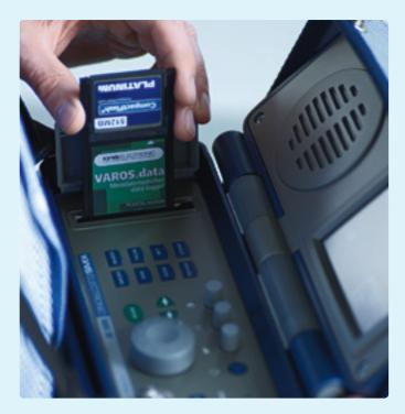
The PCMCIA modul is inserted with the CompactFlash card in the CI slot of the VAROS 307. The VAROS 307 recognizes this modul and is ready for measuring.
