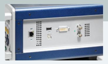
**All interface in review:** Ethernet RJ 45, ASI in/out over BNC, USB-A, USB-B, SCART, DVI out.
