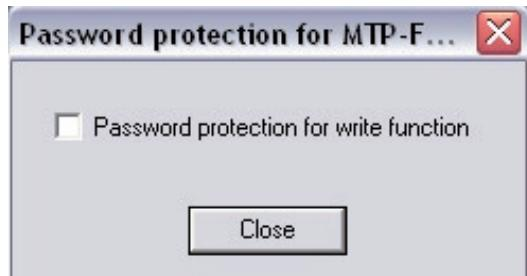
After activation of password protection the user is requested to enter the password. This password must consist of a max. 6 characters.
